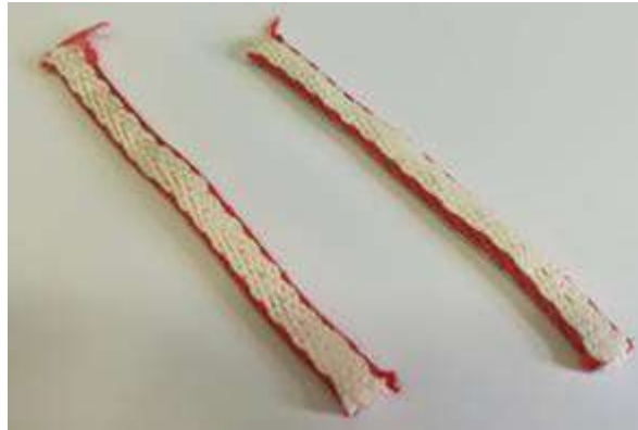
Figura 52 New and exposed Mammut Contact Sling (2 months).
