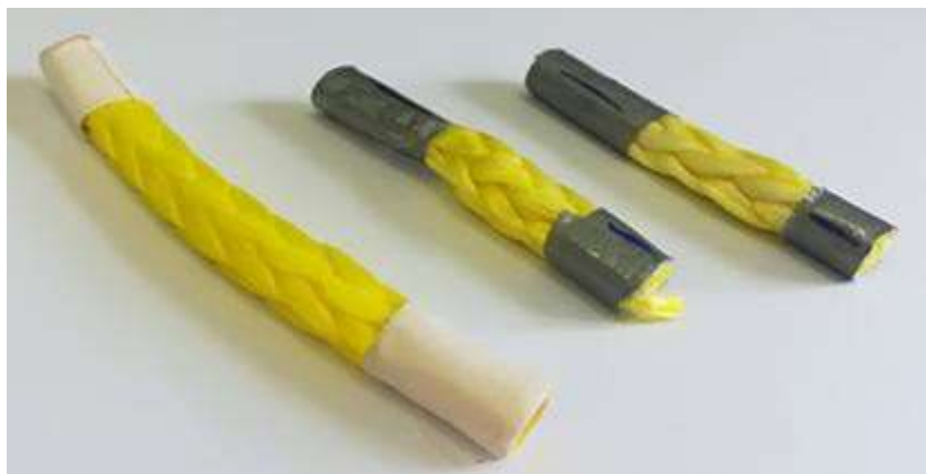
Figura 21 New and exposed samples (two and three months)
