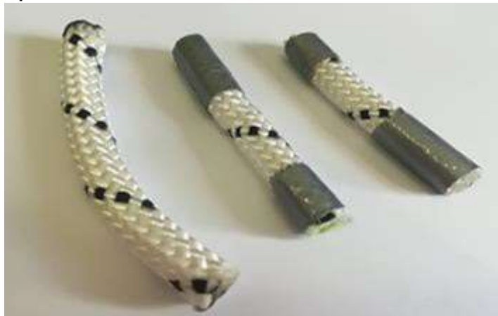
Abbildung 29 New and exposed Nylon Static samples (two and three months)
