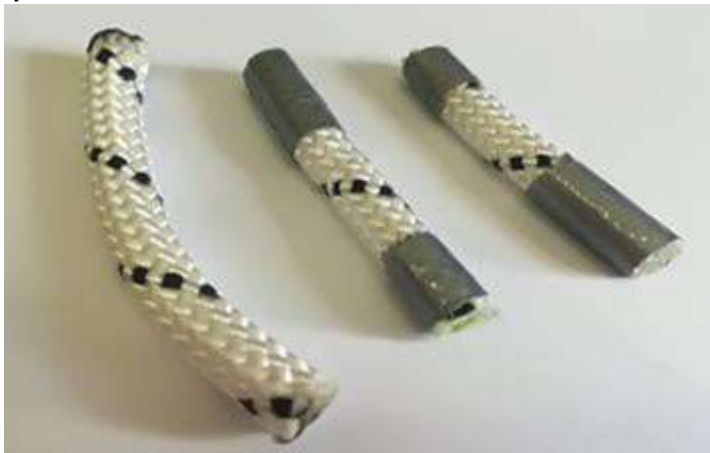
Figura 29 New and exposed Nylon Static samples (two and three months)
