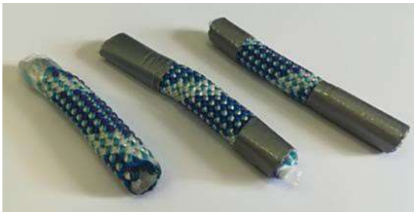
Abbildung 36 New and exposed Dynamic Classic samples (two and three months).
