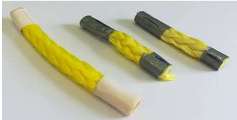
Abbildung 21 New and exposed samples (two and three months)
