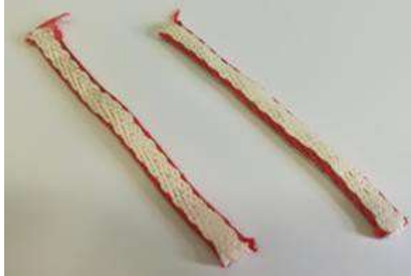
Abbildung 52 New and exposed Mammut Contact Sling (2 months).
