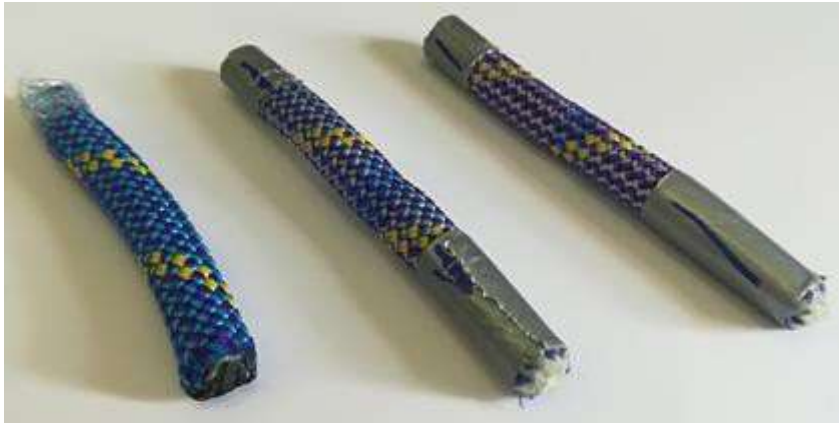
Figura 44 New and exposed Dinamic Dry samples (two and three months).
